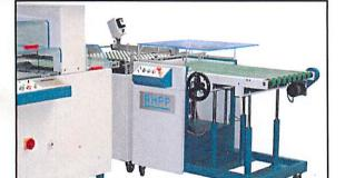
This set insure a reception of a simple pile as well of few piles side to side of pads counted, the computerized preselection insure the cadenced advance of the piles onto the conveyor of the RHPP.
